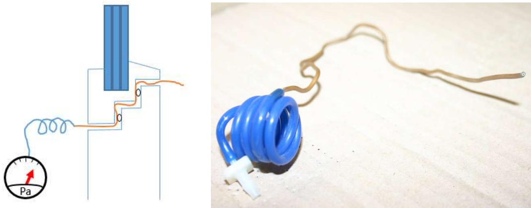
Figure 6: Capillary tube with hose connection for pressure difference measurement through a window seal (e.g. for measurement on the top floor).
